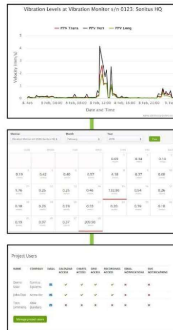
From top to bottom : data plotted over a day, calendar overview, user right permissions
